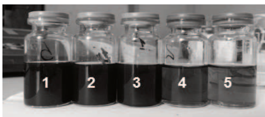
Fig. 3. Dispersions of MWCNT in DMFA: 1-; modified with PVP K-15; 2 - native + PVP K-15; 3 - native; 4 - modified with PEG 400; 5 - modified with PEG 4000.
